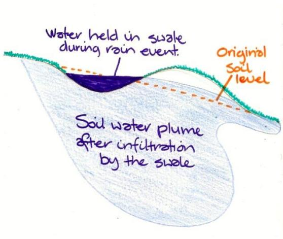
As the water runoff sits in the swale, it drops sediments and nutrients as the water is sitting relatively still. Surplus water can leave the swale over its spill way leaving behind most of what it is carrying.
